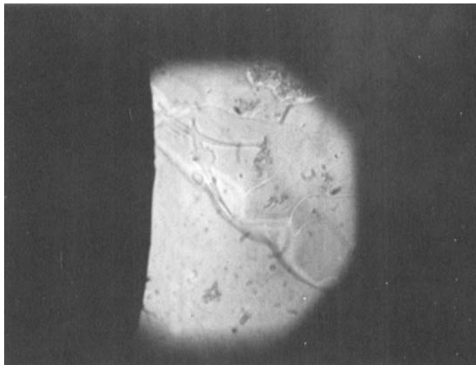
FIG. 1. Freon wash-off dissolution front of plasma fluorocarbon deposit.
